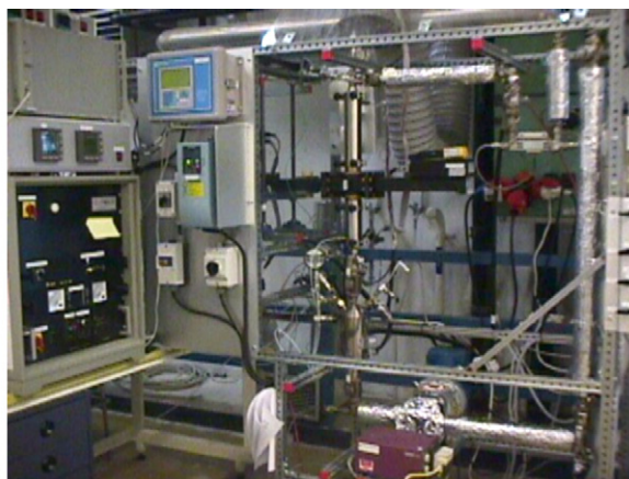
Fig. 3. (a) Schematic flow sheet of single-mode microwave loop reactor. (b) Single-mode microwave loop reactor.
